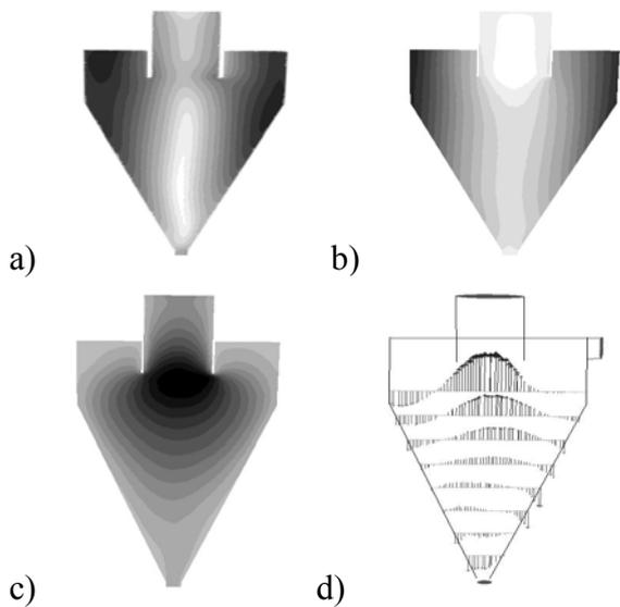
Figure 3. Contours of a) velocity b)static pressure, c)turbulent kinetic energy, d)velocity vertical vectors.
