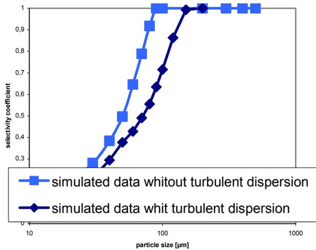
Figure 6. Simulated separation curves without and with turbulent dispersion.
